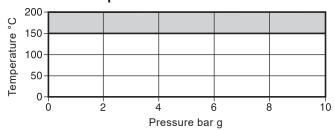
The CVS10 with EPDM seats must not be used in this region.
